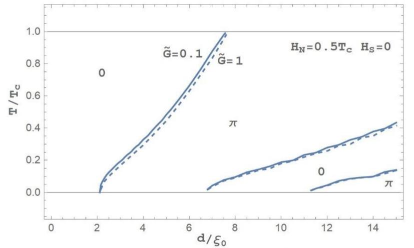
Figure 1 : calculated phase diagram of a junction in (d, T) coordinates.
