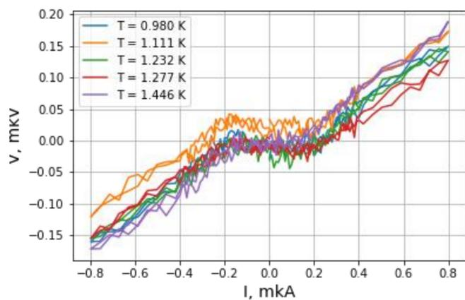
Figure 4 : example of IV characteristics of a sample
