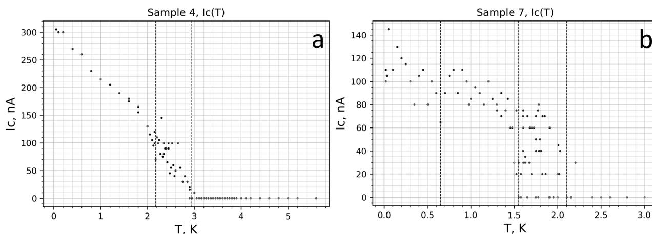
Figure 5 : critical current on temperature dependence for samples 4 (a) and 7 (b).
