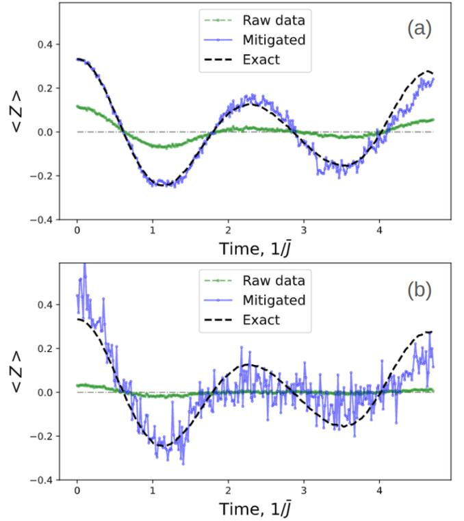
Figure 3: The dependence of a mean magnetization in  $z$  direction  $\langle Z \rangle$  of 9-spin system on time for Trotter layer numbers  $N_2 = 32$  (a),  $N_2 = 64$  (b) starting from the initial condition  $|000111000\rangle$  at  $\hbar = 2\bar{J}$ .
