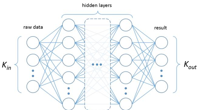
Figure 1: The schematic view of the DNN structure. The number of input (output) neurons is  $K_{in}$  ( $K_{out}$ ). Several hidden layers can be used. In our illustrative simulations we used three hidden layers each consisting of 1000 neurons. The sigmoid activation function after both hidden and output layers is utilized, while ReLU activation function is used for hidden layers.
