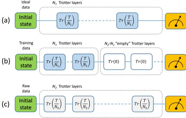
Figure 2: Schematic view of the method. (a) - Generation of ideal or quasi-ideal data using classical computation or the same quantum computer corresponding to  $N_1$  Trotter layers and different initial conditions. (b) - DNN training by adding  $N_2 - N_1$  "empty" Trotter layers to the quantum circuit and transforming such noisy data towards their ideal counterparts. (c) - applying DNN to the noisy data corresponding to  $N_2$  Trotter layers.
