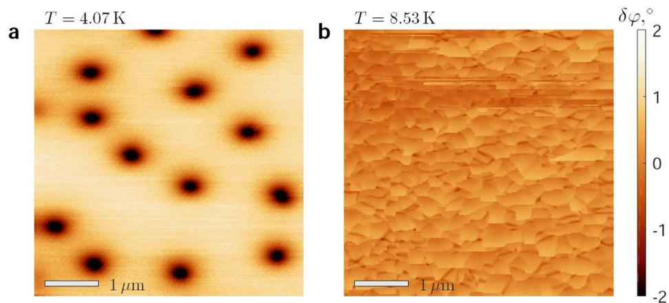
Fig.1. a – Map of the phase shift  $\delta\phi(x,y)$  acquired for 240-nm thick Nb film in the MFM regime (low- $T$  limit,  $5\times 5\ \mu\text{m}^2$ , cooled at 10 Oe, lift 80 nm). b – Map of the phase shift acquired for the same film in the SQVM regime (high- $T$  limit,  $5\times 5\ \mu\text{m}^2$ , zero magnetic field, lift 80 nm).
