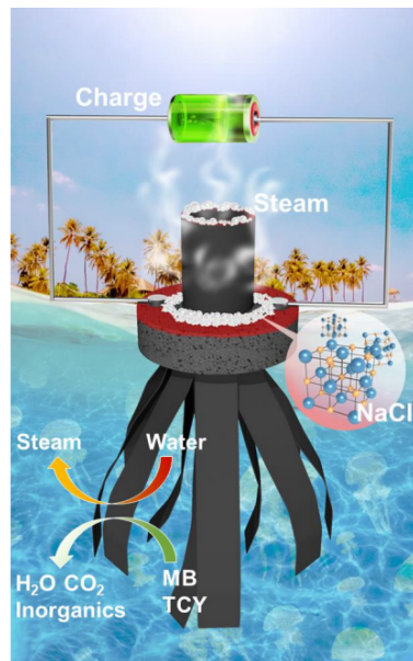
Figure 1: Multifunctional integrated 3D asymmetric nanofluid solar photothermal evaporator for seawater desalination, salt collection, power generation, and photocatalytic degradation.
