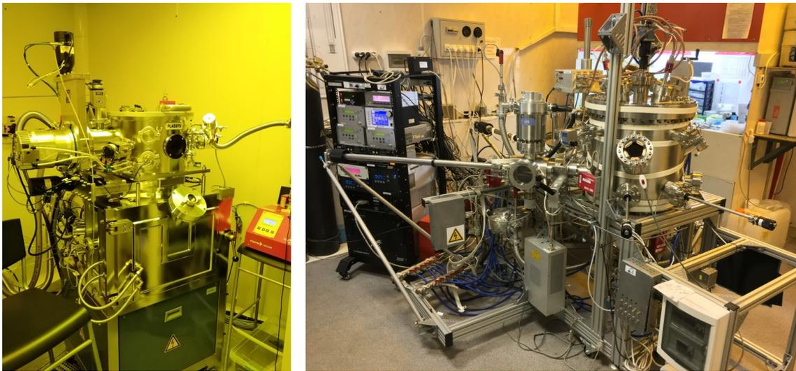
Figure 7: Left — electron beam sputtering system Plassys MEB 550 S. Right — custom developed magnetron sputtering setup
