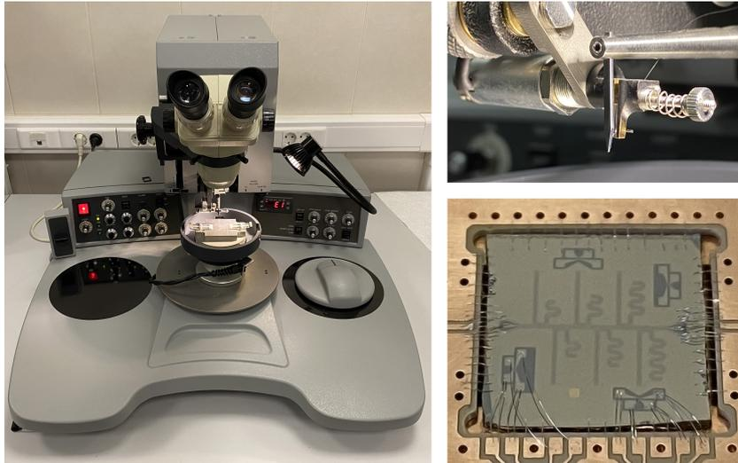
Figure 13: Ultrasonic micro-welding setup (left); a needle with aluminum thread for bonds (top right); a chip in the sample holder connected to the pads by bonds
